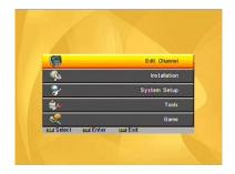
During the installation the OK key confirms a selection and LIST key shows Down List Box if the column has < > mark. You can also use the numeric keys on the RCU to enternumeric value.
